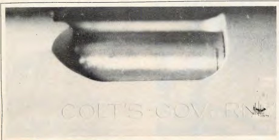
Ejection port is enlarged and shaped to facilitate positive ejection of spent cases.
